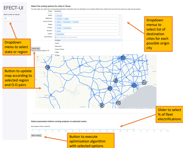
Fig. 3. A screenshot of the EFECT-UI developed to identify optimal charging locations, estimates of total energy costs, and potential reduction to emissions. Users select a region, cities for O-D pairs, and analysis parameters before executing the algorithm. Maps for the road network and selected routes are displayed.
