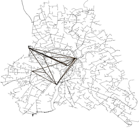
Fig. 6. The MV distribution grid of Toulouse (thin) with its minimum DG-kernel (thick).
