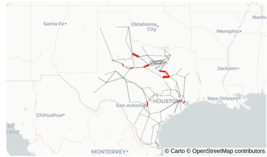
Fig. 6. Baseline TNEP Investments. Red lines indicate the location of capacity upgrades, with the thickness/width of each line representing one of the three available upgrade levels.
