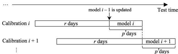
Fig. 6. Recalibration strategy: the model  $i-1$  is updated with the information from the  $r$  previous days to obtain model  $i$ , which is then used for the actual day-ahead predictions for each of the next  $p$  days. Then, the model  $i$  is updated using data from the  $r$  past days (to obtain model  $i+1$ ), and the same procedure is carried out over time.
