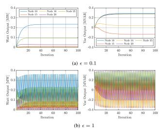
Fig. 3. Evolution of active and reactive power setpoints under the proposed power update rule (6) with (a)  $\epsilon = 0.1$  and (b)  $\epsilon = 1$ , where we use the power data profiles of the 1095-th minute and consider 100 iterations.
