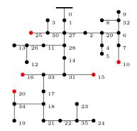
Fig. 1. IEEE 37-bus feeder. Red nodes represent buses hosting DERs, black nodes represent loads.
