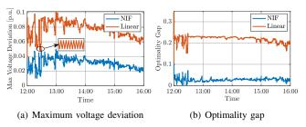
Fig. 4. Maximum voltage deviation and optimality gap with respect to the OPF solutions along the evolution. The linear control method induces instability between 12:00 and 13:00.
