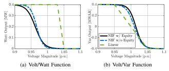
Fig. 2. Learned (a) Volt/Watt and (b) Volt/Var curves for node 25 using 795th minute-based load and generation profiles with and without equity design.
